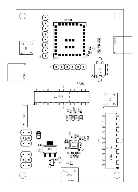
Figure 10: Reference design: Assembly diagram
