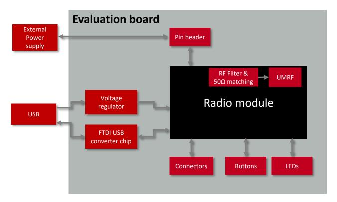
Figure 3: Block diagram
