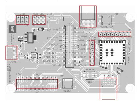
Figure 5: Connector and pin headers
