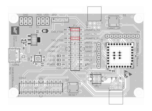
Figure 7: Application UART connected to USB communication
