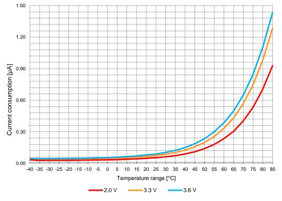
Figure 3: Current consumption during Sleep mode
