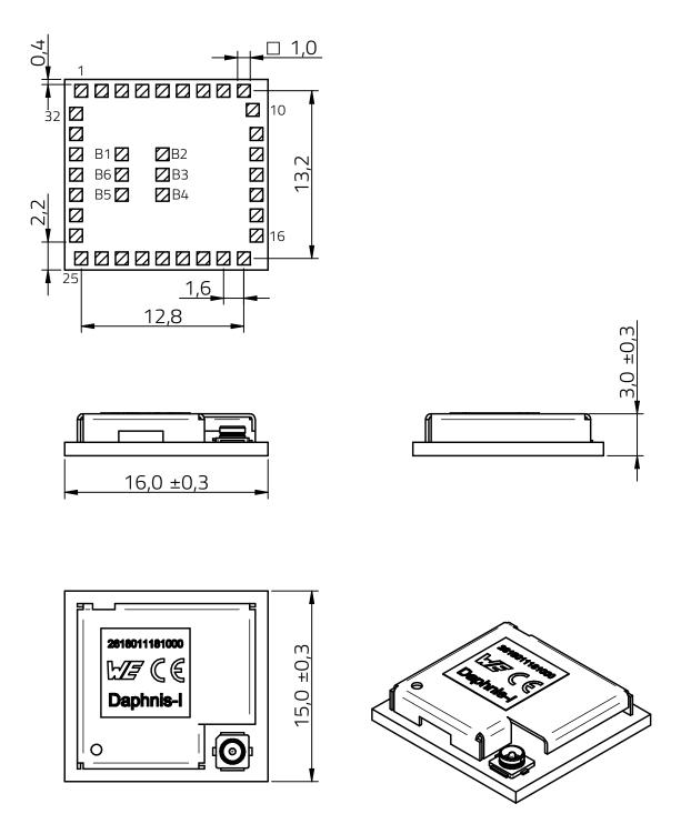
Figure 44: Module dimensions [mm]
