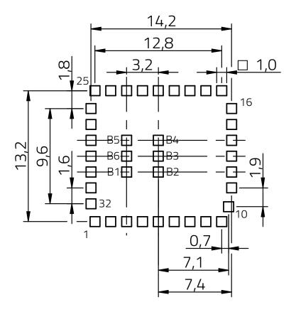
Figure 45: Footprint and dimensions [mm]
