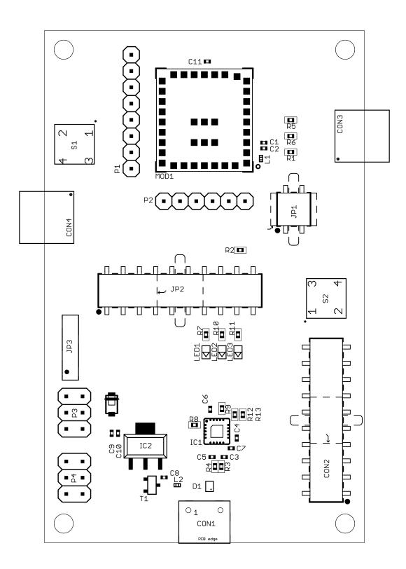
Figure 41: Reference design: Assembly diagram
