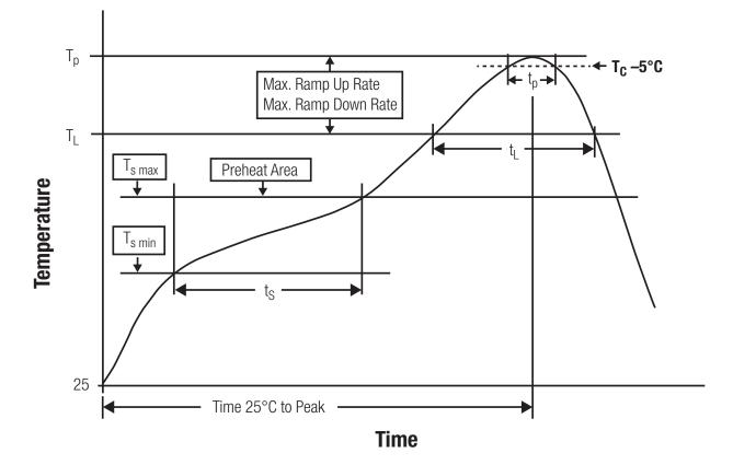
Figure 43: Reflow soldering profile
