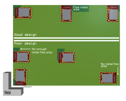
Figure 35: Placement of the module with integrated antenna
