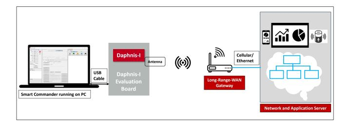
Figure 15: Daphnis-I quick start setup
