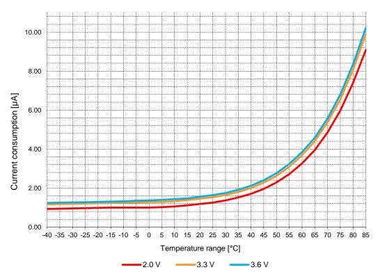
Figure 4: Current consumption during Idle state
