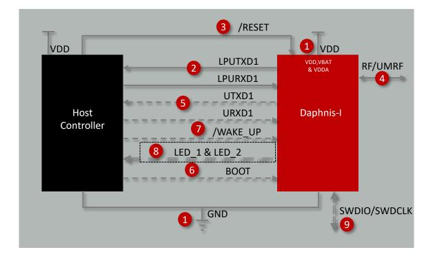
Figure 13: Minimal pin connections
