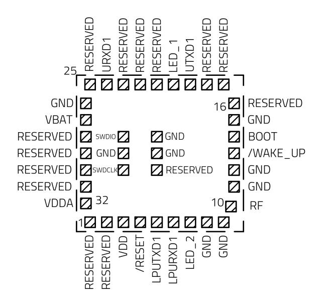
Figure 5: Pinout (top view)
