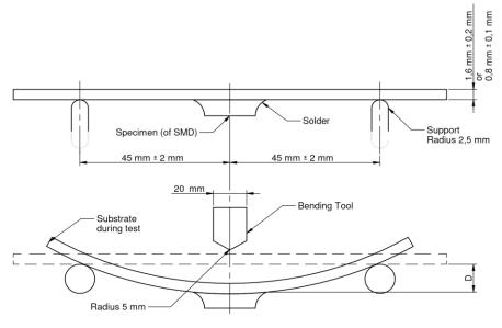
This substrate bending test is for all size of WCAP-CSST.
