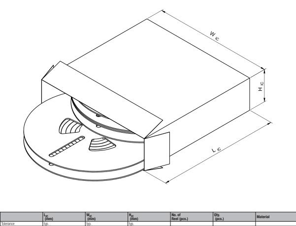
C т W vc С No. of Qty. (pcs.) L<sub>C</sub> (mm) Material (mm) (mm) Inner Carton (pcs.) Tolerance typ. tvp typ. Value 425.00 412.00 340.00 3600 Paper CHECKED REVISION DATE (YYYY-MM-DD) GENERAL TOLERANCE PROJECTION METHOD (⊕) FPu 002.000 2022-09-14 DIN ISO 2768-1m DESCRIPTION TECHNICAL REFERENCE WCAP-PSLC Aluminum Polymer PSEF124181M035DVCTFB000 Würth Elektronik eiSos GmbH & Co. KG **Capacitors** ORDER CODE 875075661007
