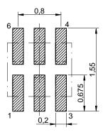
PCB Design: To simplify the routing, is possible to place a trace connecting the pads (1 & 6) (2 & 5) (3 & 4) Scale - 20:1
