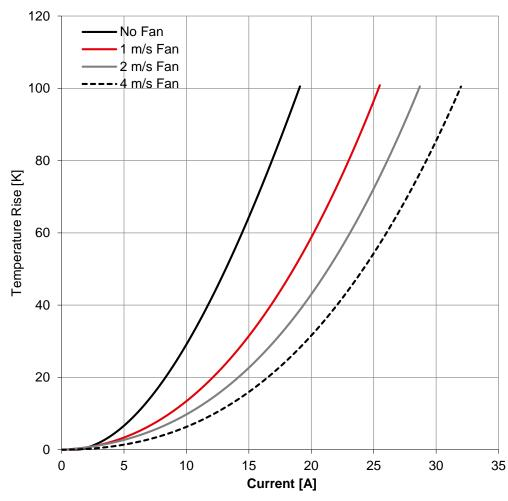
Airflow testing was done with 115mm Ø fan and air velocity was measured directly in front of the part between the fan and part.
