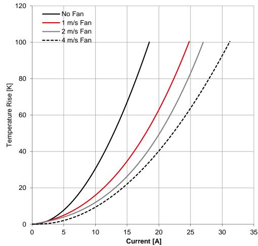
Airflow testing was done with 115mm Ø fan and air velocity was measured directly in front of the part between the fan and part.
