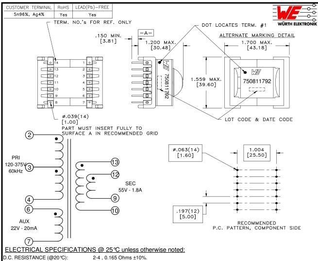
6-7, 0.132 Ohms ±10%. 9-12 , 0.115 Ohms max. 10-13, 0.115 Ohms max.
