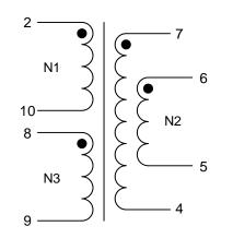
N2 denotes two windings connected in parallel. Terminals 4+5 and 6+7 must be tied as solder bridging is allowed.
