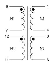
Customer to tie terminals 1&3 and 4&6 internally on the PC Board.
