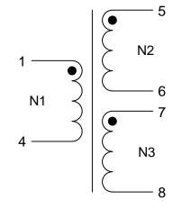
Application of the transformer allows for the leadwires between terminals 6&7 to solder bridge.
