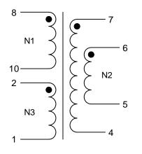
N2 denotes two windings connected in parallel. Terminals 4+5 and 6+7 must be tied as solder bridging is allowed.
