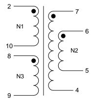
N2 denotes two windings connected in parallel. Terminals  $4\!+\!5$  and  $6\!+\!7$  must be tied as solder bridging is allowed.
