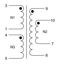
Application of the transformer allows for the leadwires between terminals 6&7 and 9&10 to solder bridge.
