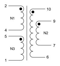
Customer to tie 6&7 and 9&10 on PCB board. Application of the transformer allows for the lead wires between terminals 6&7 and 9&10 to solder bridge.
