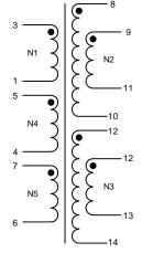
Customer to tie terminals 8&9, 10&11 and 13&14 on PC board. Application of the transformer allows for the leadwires between terminals 8&9, 10&11 and 13&14 to solder bridge.
