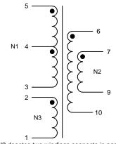
N2 denotes two windings connecte in parallel. Terminals 6+7, 9+10 must be tied as solder dridging is allowed.
