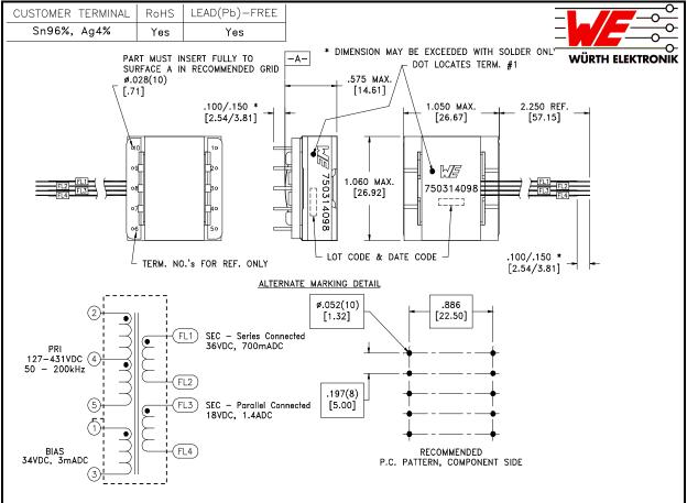
Designed for total output power of 25 Watts.
