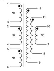
N3 denotes three windings connected in parallel. Terminals 7 + 8 + 9and 10 + 11 + 12 must be tied as solder bridging is allowed. Terminals 2 + 3 must be tied as solder bridging is allowed.
