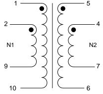
N1, N2 denotes two windings connected in parallel. Terminals 1+2, 9+10, 4+5 and 6+7 must be tied as solder bridging is allowed.
