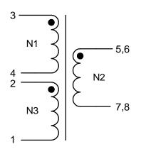
Application of transformer allows for leadwires between terminals 7&8 to solder bridge.
