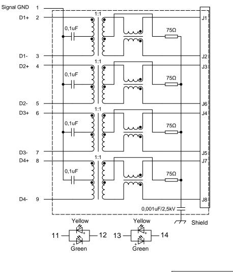
CHECKED REVISION DATE (YYYY-MM-DD) GENERAL TOLERANCE PROJECTION METHOD JefL 001.000 2021-04-07 DIN ISO 2768-1m 9 DESCRIPTION RoHS COMPLIANT REACh WE-RJ45 LAN Transformer Würth Elektronik eiSos GmbH & Co. KG ORDER CODE EMC & Inductive Solutions Max-Eyth-Str. 1 74991104404 74638 Waldenburg Germany Tel. +49 (0) 79 42 945 - 0 www.we-online.com STATUS BUSINESS UNIT PAGE WÜRTH ELEKTRONIK 2/6 eiSos Valid eiSos@we-online.com
