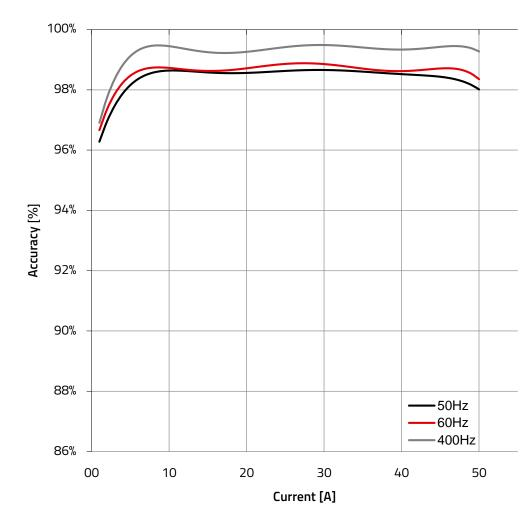
Response testing was completed with a burden resistor value of  $66.66\Omega$  to achieve a 1V output at 45A
