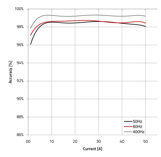
Response testing was completed with a burden resistor value of  $55.55\Omega$  to achieve a 1V output at 45A
