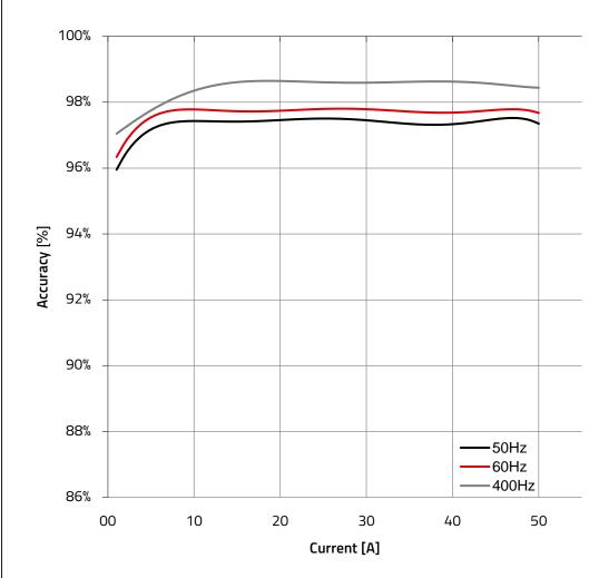
Response testing was completed with a burden resistor value of  $22.22\Omega$  to achieve a 1V output at 45A
