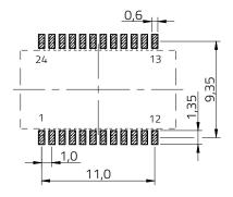
Unless otherwise defined tolerance: ±0,10mm no vias or traces underneath the component
