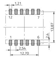
Unless otherwise defined tolerance: ±0,10mm no vias or traces underneath the component
