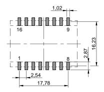
no vias or traces underneath the component Scale - 1,5:1
