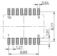
Unless otherwise defined tolerance: ±0,10mm no vias or traces underneath the component
