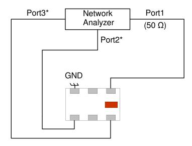
\*Impedance for ports 2 and 3=1/2(Balanced impedance)
