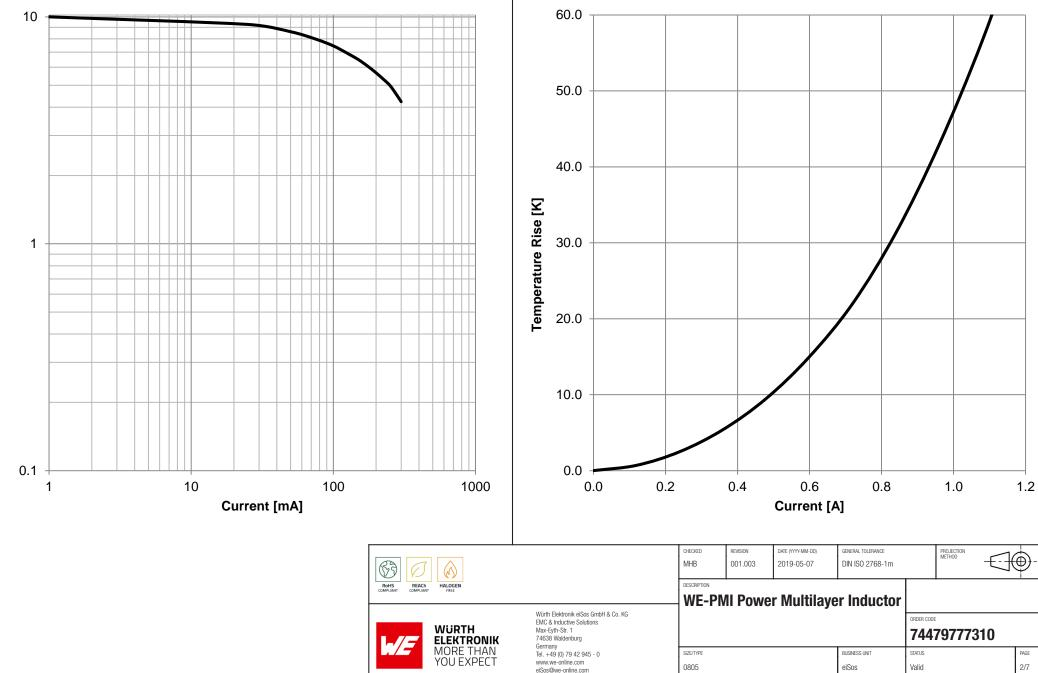
**Typical Temperature Rise vs. Current Characteristics:**
