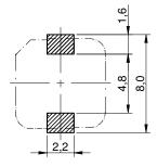
no sensitive traces underneath the component
