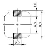
no sensitive traces underneath the component
