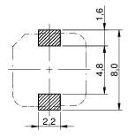
no sensitive traces underneath the component
