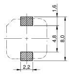
no sensitive traces underneath the component
