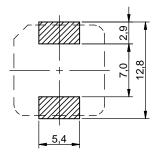
no sensitive traces underneath the component
