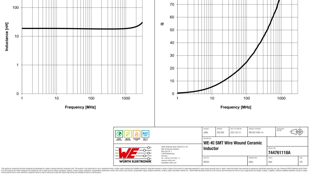
**Typical Inductance vs. Frequency Characteristics:**
