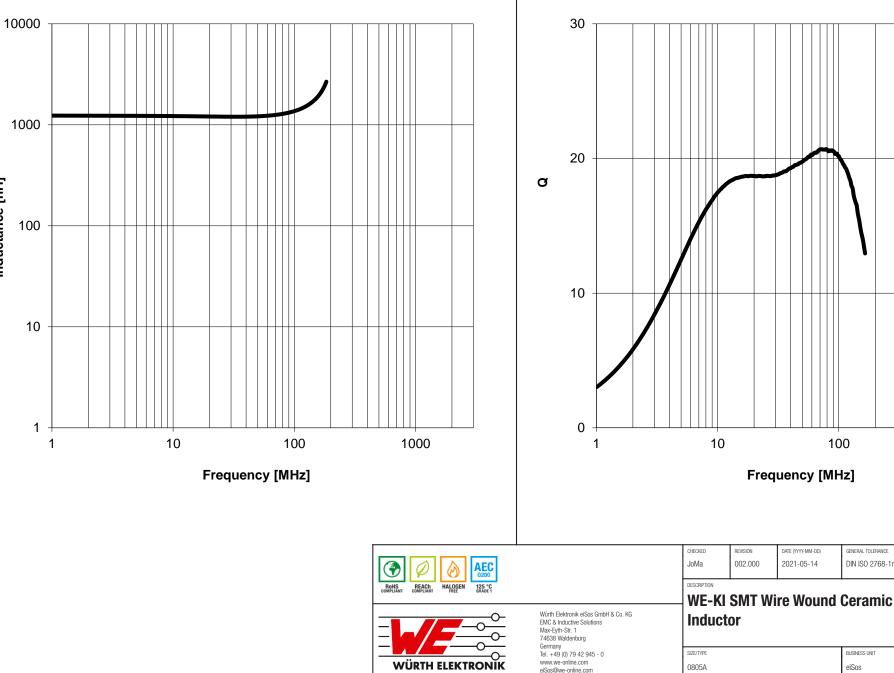
**Typical Inductance vs. Frequency Characteristics: Q-Factor vs. Frequency:**
