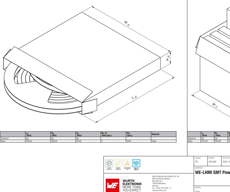
No. of Qty. (pcs.) (mm) Material Inner Carton (pcs.) typ. 354.00 16000 Paper DATE (YYYY-MM-DD) GENERAL TOLERANCE PROJECTION METHOD  $\oplus$ 2024-12-27 DIN ISO 2768-1m **WE-LHMI SMT Power Inductor** ORDER CODE 74437336068
