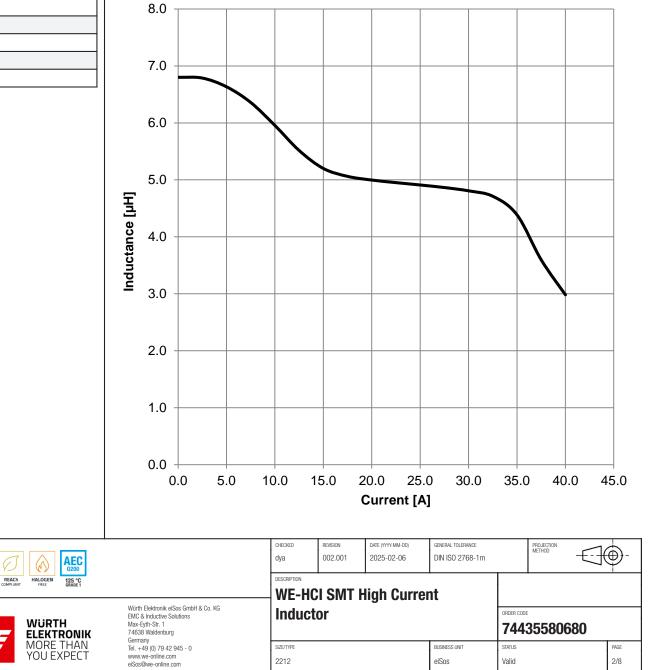
This electronic component has been designed and developed for usage in general electronic equipment only. This product is not authorized for use in equipment where a higher safety standard and reliability standard and rel
