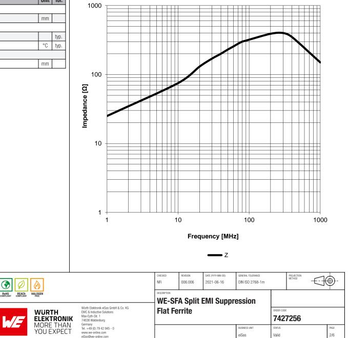
This electronic component has been designed and developed for usage in general electronic equipment only. This product is not authorized for use in equipment where a higher safety standard and reliability standard and rel
