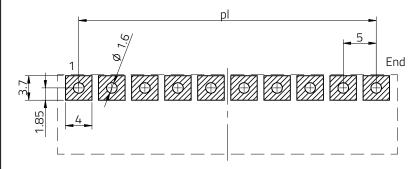
Stencil thickness: 120 µm
