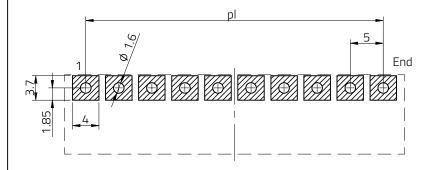
Stencil thickness : 120 µm
