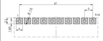
Stencil thickness: 120 µm
