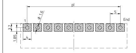
Stencil thickness: 120 µm
