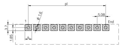
Stencil thickness: 120 µm
