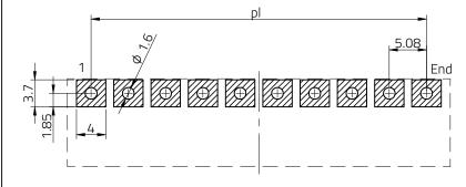
Stencil thickness: 120 µm
