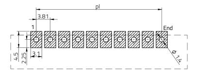
Stencil thickness: 120 µm
