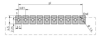
Stencil thickness: 120 µm
