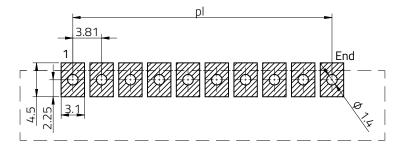
Stencil thickness: 120 µm
